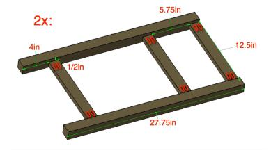
Clamp the 2x2x27.5" to the 1x2x12.5" board (sandwiched between your ½" and ¼" spacers) and glue and screw together, as shown below with 1-¼" pocket hole screws. Make sure to wipe off any excess glue (Hint: Glue doesn't stain).
