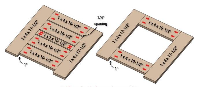
Drill pocket holes and assemble front and back using 1-1/4" pocket screws
