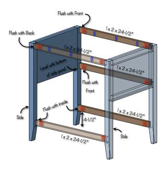
Drill pocket holes in the five  $1 \times 2 \times 24$ -1/2" boards. Pocket holes shown in blue will be used to fasten the top in the next step.
