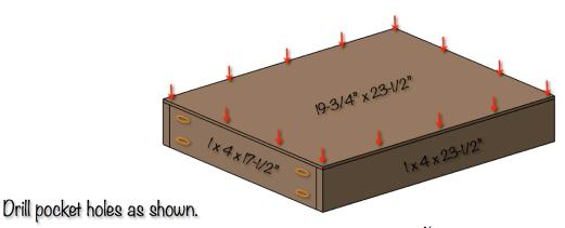
Then assemble box using 1-1/4" pocket hole screws and 1-1/4" brad nails.
