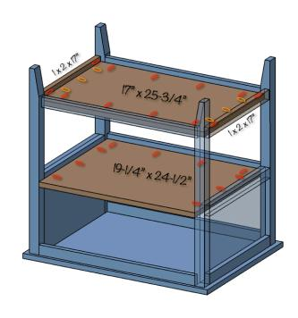
Orill pocket holes in all boards as shown.
