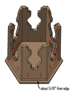
Using pre-existing pocket holes from the previous step, attach the base to the top using I-I/4" pocket screws
