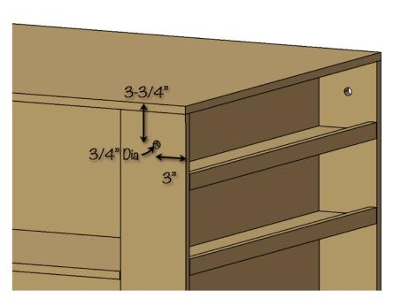
If you would like to install a roll of Rosin paper to protect your work surface as I have, you will need to drill a 3/4" hole as shown to accept the rod.
