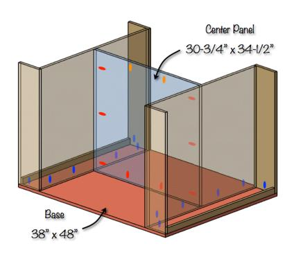
Drill pocket holes as shown in the center panel.
