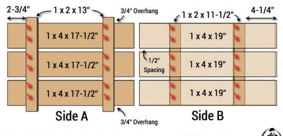
Assemble 4 of each, sides A and B, as shown using 1-1/4" wood screws.
