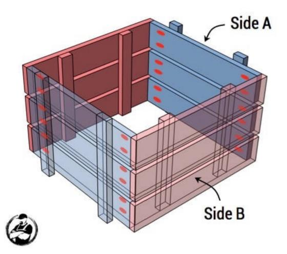
Drill pocket holes and assemble crates (qty 2) as shown using 1-1/4" pocket hole screws.
