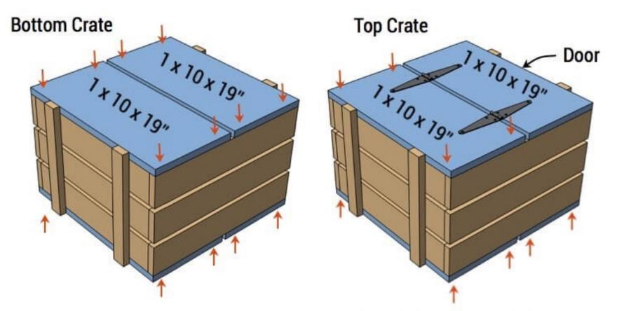
Install tops and bottoms using 1-1/4" wood screws. Then install hinges using hardware included.
